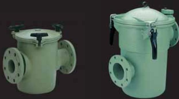
Housing and cover in cast iron. AISI-304 stainless steel strainer basket. Flange connection are manufactured in accordance with DIN-2501 Standard. Maximum working pressure 2.5 bar.
