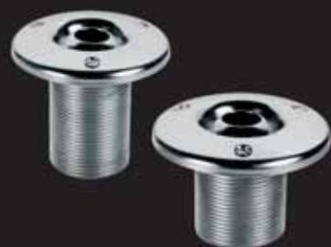
Outer 1 1/2" thread. Made of AISI-316 stainless steel. Max. recommended flow rate compliant with standard EN 13451-3: 4.5 m<sup>3</sup>/h. Ø 20 mm eyeball.
